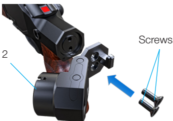
Pic. 29 Folding unit 2 is installed.
