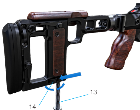
Pic. 23 Monopod adjustment.
