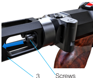
Pic. 24 Unscrew the screws.
