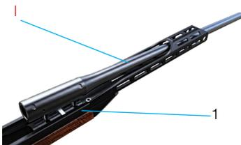
Pic. 9 Install the barrel
