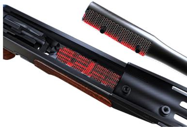
Pic. 85 Marked area must be degreased
