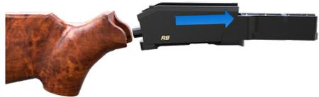
Pic. 27 Remove the buttstock.
