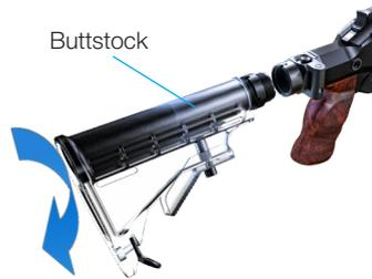
Pic. 72 Install the buttstock.
