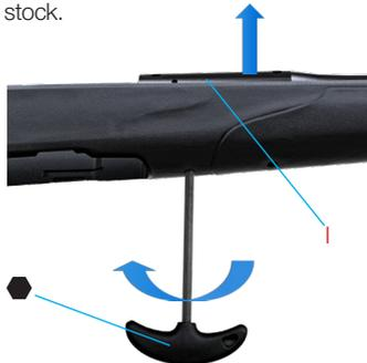
Pic. 8 Remove the barrel
