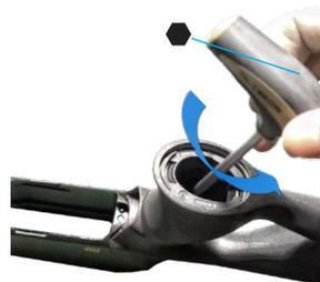
Pic. 23 Remove the lower fixing screw.
