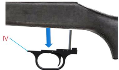
Pic. 43 Remove the trigger.
