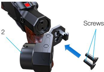
Pic. 69 Folding unit 2 is installed.
