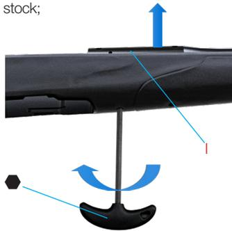
Pic. 41 Remove the barrel.
