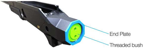
Pic. 34 Install the Threaded bushing and the End Plate.
