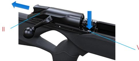
Pic. 7 Remove the bolt
